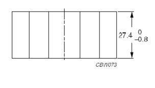
**E cores** are mainly used in power transformers. Below are examples of cores materials we use for the manufacture of our products. These cores occur with different slots and AL values. AL values are given for cores without slots. For our production we also use cores with different slots of different constant AL eg: 630, 400, 315, 250, 160, 100 as well as other made according to individual customer requirements.
