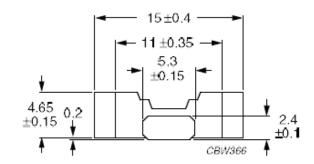
**FFD cores** are particularly applicable in low power transformers, thanks to the untypical design - flattened center column, placed asymmetrically. Thanks to this we get compact construction and lowered transformer height in comparison to a similar power transformer on the EE core. Below are examples of core materials we use for the manufacture of our products.
