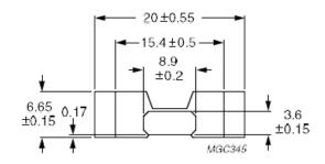
**FFD cores** are particularly applicable in low power transformers, thanks to the untypical design - flattened center column, placed asymmetrically. Thanks to this we get compact construction and lowered transformer height in comparison to a similar power transformer on the EE core. Below are examples of core materials we use for the manufacture of our products.
