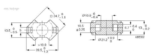
**RM cores** are mainly used in Telecommunication and pulsed transformers, where galvanic separation is required, as well as in chokes and coils and resonant circuits. The shape of the cores enables optimal use of the winding space with very good magnetic shielding.Below are examples of core materials we use for the manufacture of our products. These cores occur with different slots and AL values.
