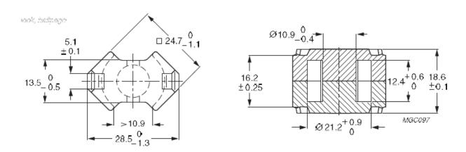
**RM cores** are mainly used in Telecommunication and pulsed transformers, where galvanic separation is required, as well as in chokes and coils and resonant circuits. The shape of the cores enables optimal use of the winding space with very good magnetic shielding.Below are examples of core materials we use for the manufacture of our products. These cores occur with different slots and AL values.
