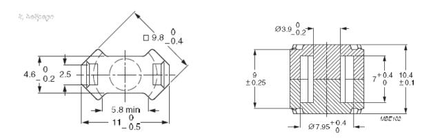
**RM cores** are mainly used in Telecommunication and pulsed transformers, where galvanic separation is required, as well as in chokes and coils and resonant circuits. The shape of the cores enables optimal use of the winding space with very good magnetic shielding.Below are examples of core materials we use for the manufacture of our products. These cores occur with different slots and AL values.
