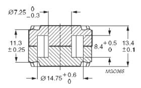
**RM** cores are mainly used in Telecommunication and pulsed transformers, where galvanic separation is required, as well as in chokes and coils and resonant circuits. The shape of the cores enables optimal use of the winding space with very good magnetic shielding. Below are examples of core materials we use for the manufacture of our products. These cores occur with different slots and AL values.
