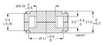
**RM cores** are mainly used in Telecommunication and pulsed transformers, where galvanic separation is required, as well as in chokes and coils and resonant circuits. The shape of the cores enables optimal use of the winding space with very good magnetic shielding. Below are examples of core materials we use for the manufacture of our products. These cores occur with different slots and AL values. AL values are given for cores without slots.
